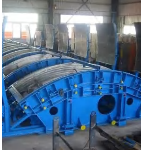
Prefabricated Tunnel Segment Mold
