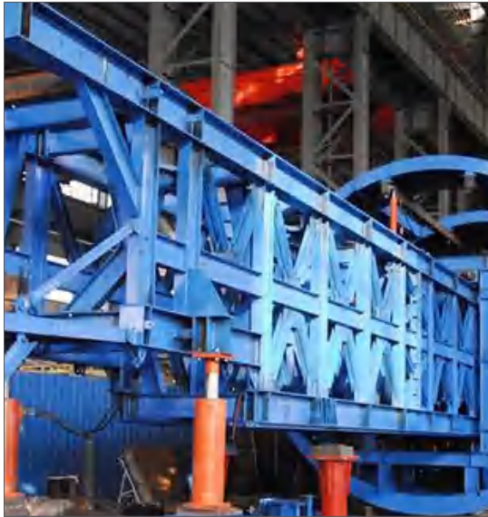
Circle Tunnel Needle Beam Trolley
